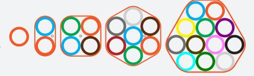
Höhle microducts are designed for long term protection of fiber optical cables. Direct Bury (DB) type of microducts are thick wall products that attain their mechanical robustness and functional performance through their intrinsic thick walls and need no further protection at underground installations. Höhle microducts conform to BS FN 61386 and BS FN 60794-5.
